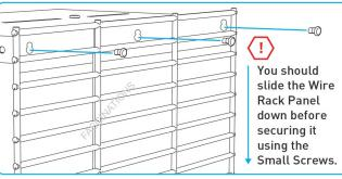
Drive the screws halfway into the Top and Bottom Attachment Squares first, then hang the panel and tighten the screws.
